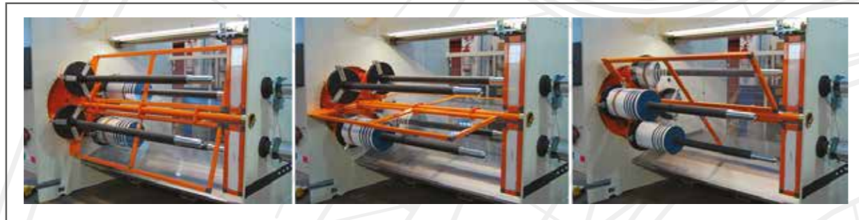
Automatic management of the turret shafts revolving system, checked by PLC and servo motors
