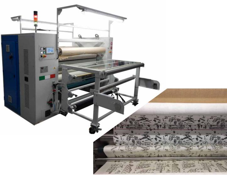
Laminator machine for laminating and sublimation transfer printing working width 1800 mm, max material width 1600 mm. Hot calander roller ø 350 mm with working temperature up to 230° C (464° F), Blast chiller roller to drop down temperature of the materials to fixing and secure printing or bonding results. Independent pressure controll, automatic alignment of the calender felt, Protective Paper to save the calender felt, wide range configuration with pull-out table or unwinders,
