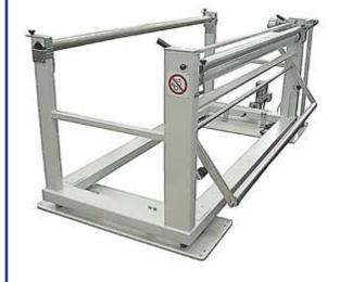
Roll holder with stainless steel shaft, roll holding flanges and mechanical brake, equipped with a motorized feeding entry calander, composed by metal or silicone rollers with handles and
